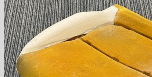
After taking the normal section templates, cut the defective area and repair them with urethane blocks of the same density as the original.
