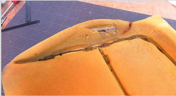
In the case of the urethane foam is torn off and the frame is exposed.
