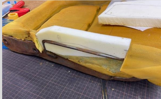
After taking the normal section templates, cut the defective area and repair them with urethane blocks of the same density as the original.
