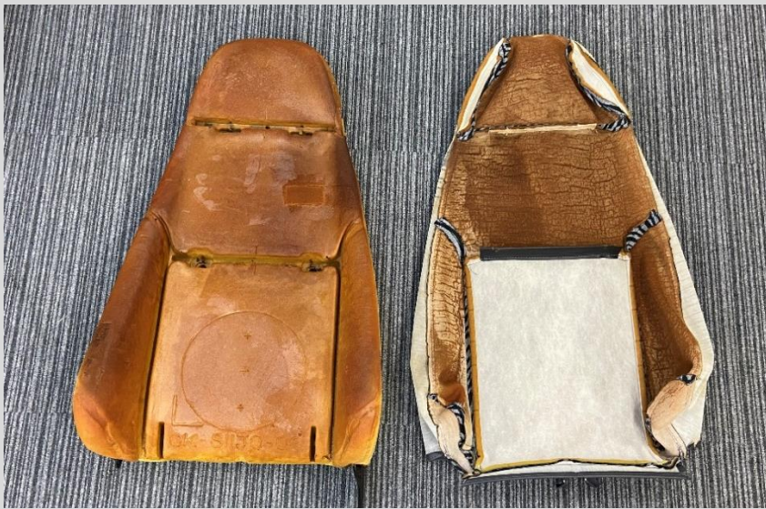
The old trim cover has been removed.
