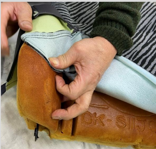
Covering along the groove.
