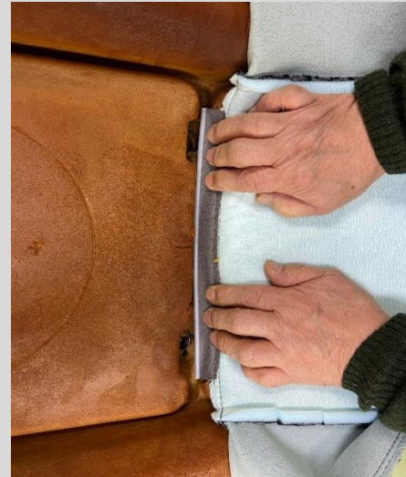
Put on the new trim cover and fasten it in the reverse order of the removal of the old trim cover: apply C-rings to the listing wire of the lower part of the headrest, and then the center part.
