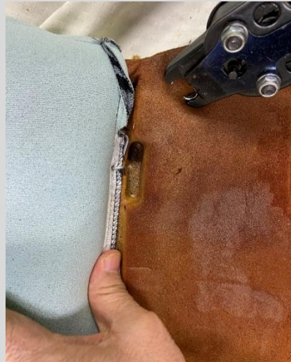
Put on the new trim cover and fasten it in the reverse order of the removal of the old trim cover: apply C-rings to the listing wire of the lower part of the headrest, and then the center part.
