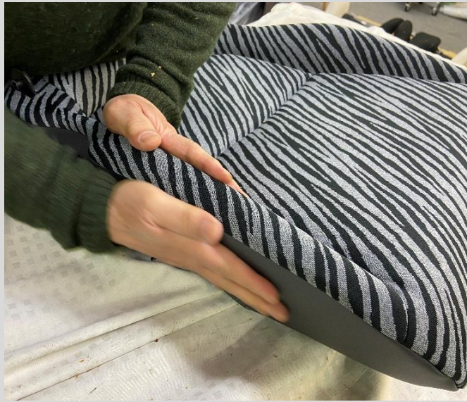
Adjust the shape by hand checking the location of the seam edge inside.
