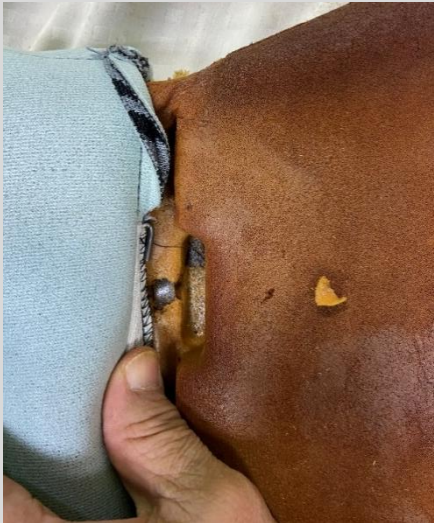
Put on the new trim cover and fasten it in the reverse order of the removal of the old trim cover: apply C-rings to the listing wire of the lower part of the headrest, and then the center part.
