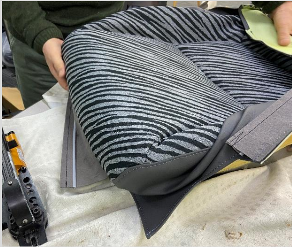
After finishing the covering, clip the back side all the way around. Pull hard on the trim cover to keep it from sagging.
