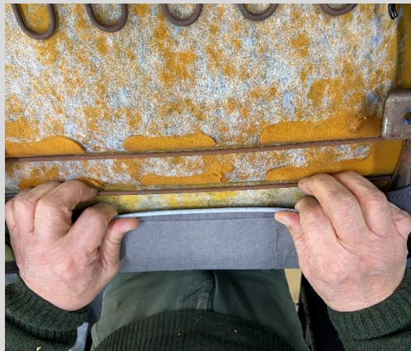
After finishing the covering, clip the back side all the way around. Pull hard on the trim cover to keep it from sagging.
