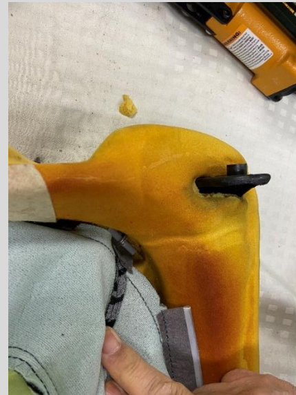
Next, fasten all the way around the side bolsters and the listing area of the cushion.
