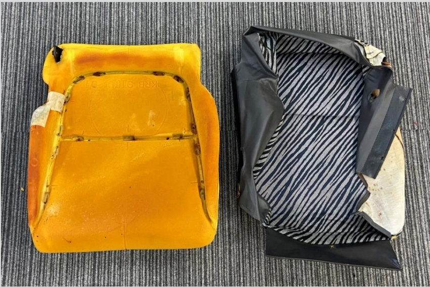
Now, old trim cover is removed.
