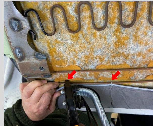
After finishing the covering, clip the back side all the way around. Pull hard on the trim cover to keep it from sagging.
